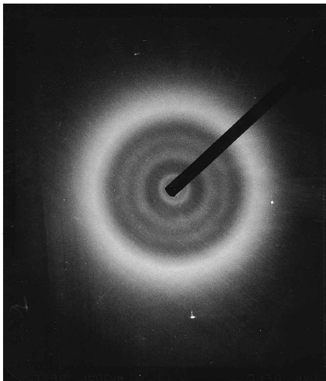
Figure 1. Example of a pin-hole camera powder X-ray diagram of the azo-substituted poly(L-lysine) Azo-Lys-41 containing 41 mol% of azobenzene units and showing the three sharp reflections and the diffuse band.
